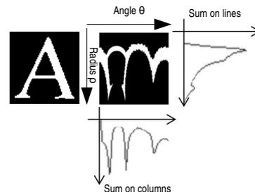
**Fig. 3** From Cartesian coordinates to 1D signal. Left: the original letter. Middle: its representation into the  $(\rho, \theta)$  space. Summation of lines (right) and columns (bottom) of polar image.
