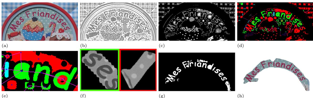
**Fig. 1** Steps of our chain at one scale and with one polarity (a) Input image (b) TMMS segmentation (c) Geometric filters (d) Shape analysis (e) Zoom on graph grouping (f) Valid and invalid candidate text areas (g) Binarization (h) Image restricted to the precise text localization result.
