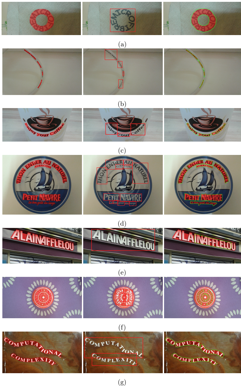
Figure 18: Examples of text areas (inclined, curved, in perspective, circular); left: mask GT annotation (red); center: rectangular GT annotation (red); right: GT masks (red) overlapped by detection masks (green). The rectangular detections are not represented but correspond to boxes surrounding the detection masks in the last column which are matched with the GT rectangles shown in the second column.
